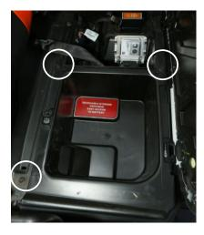
First you will need to remove the factory under seat storage compartment on the passenger side, and remove the 3 Torx bolts as shown
