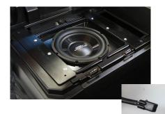
You can now place the enclosure in position under the seat and re-install the factory Torx Bolts, use the included "self-tapping" screw for the final hole location on the lower left bracket. Plug the input connector to the amp out connector from the overhead unit.
