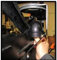
47. Slide two **SK-P-1527** (1 ½" x 10 ½" pipes) into the elbows. Then loosely slide the RIGHT riser into the corresponding clutch exhaust hose. Do not glue these into the elbows yet.
