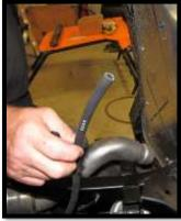
62. Insert a barbed fitting **BHF-14-ST** into the vent hose, followed by a bellow **VB01**. Use **11" zip ties** to secure the hose and bellow to the frame in a place it won't get damaged.
