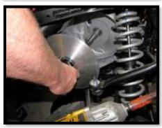
13. Remove the bolt and corresponding hardware from the primary clutch.
