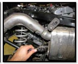
18. Once you have removed the bolts, apply silicone under the head of each one and then screw them back in. **NOTE: Do not reinstall the clutch housing cover yet.**
