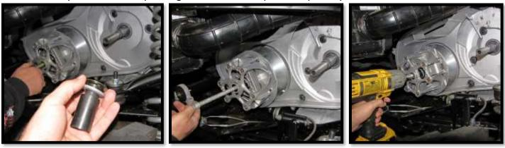
31. Reinstall the belt and secondary clutch
