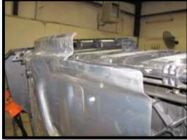
55. Find the bed plate **75L**. Center it on the bed using the large holes and where it meets the snorkels. Then trace the inside with a marker.
