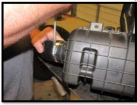
41. Reinstall the factory air box with the new air intake hose. The high lifter logo should be at the top of the hose and facing away from the cab.
