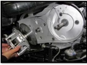
15. Remove the three bolts from the left side of the clutch housing. Apply silicone under the head of each bolt and then screw them back in.
