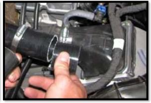
45. Next, slide the **SK-P-1506** (3" pipe) into the clutch outlet duct. Center it and slide the clutch exhaust hose on. Attach and tighten with two **HC36** hose clamps.
