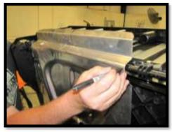
54. Trim the heat shield with a grinder where you marked it. Once finished, make sure it has proper clearance and trim extra if needed.
