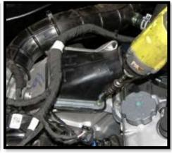
24. Apply a generous amount of silicone under and around the edges of the port inside the clutch housing. This will help ensure no water will leak in.
