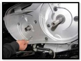
16. In the next steps, you will remove the four bolts from the right side of the clutch housing.
