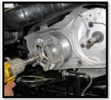
30. Use the factory bolt and corresponding hardware to complete the primary clutch installation.
