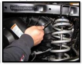
34. Insert two **27A** rubber grommets into the top holes of riser plate **75G**. **NOTE:** If you have a cab or rear window, the grommets will also prevent it from being scratched or damaged.
