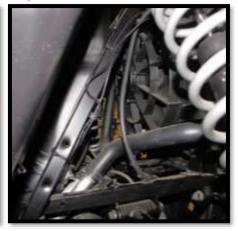
64. Find any precut holes or opening to route the vent line through to the front storage compartment. Once through, insert a barbed fitting **BHF-14-ST** into the vent hose, followed by a bellow **VB01**. Use **11" zip ties** to secure the hose and bellow in a place it won't get damaged.
