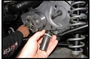
14. Use a clutch puller to remove the primary clutch.
