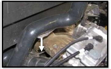
40. Next, slide the new air intake hose **75A** onto the air box inlet. Position it so that the high lifter logo is at the top of the hose and facing away from the cab when you reinstall the air box in the next step. Doing this before installing the air box will make the installation much easier and prevent having to adjust it. Attach and tighten down with hose clamp **HC40**.
