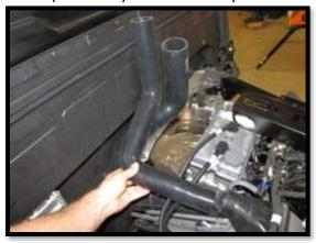
44. Once in the correct position, you may need to trim the excess hose that exceeds past the mouth of the clutch outlet duct.
