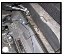
68. You can route the line through the cab frame behind the seats. If gas was to over flow from the vent line, it is necessary that it does not come in contact with the engine or exhaust. Use zip ties to secure it if needed.
