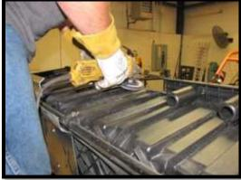
57. Gently fold the bed down to the snorkels to check clearance. Make adjustments, mark, and trim any extra plastic that's needed.
