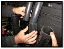
48. Loosely slide the small clutch exhaust hose **75D** onto the LEFT riser. It is very important that it be positioned (as in the picture below) so that it can blow the excess engine heat out of the engine bay. The high lifter logo should be at the top of the hose and facing away from the cab.
