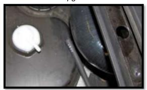
67. Insert the 5' vinyl hose **SK-VT-2** into the barbed fitting on the gas tank. You will need to route it up the cab. Drilling a routing hole in the plastic is optional. It just needs to be clear from being pinched or damaged.
