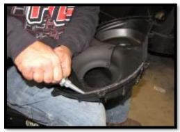
33. Reinstall the clutch housing cover and make sure it's properly sealed.
