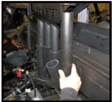
50. Once the 2" risers are lined up and you know where to trim, slide them out of the riser plate and pull them back. Use a grinder to trim the plastic lip so that each 2" riser can sit flush to the back of the cab.
