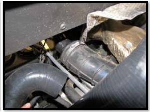
39. Insert the new clutch intake hose **75B** onto the pipe. Align the hose to the back of the cab and riser plate in the proper position. The high lifter logo should be at the top of the hose and facing away from the cab. Attach and tighten it with hose clamp **HC40**. You may need to bend the exhaust heat shield down at the edge to provide more clearance for the hose.
