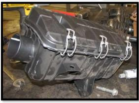
11. Remove the clutch housing cover. You will need to jack up the rear of the ranger to gain more clearance from the control arms.
