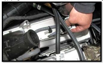
28. Before reinstalling the factory clutch inlet duct, you must insert all the factory screws back into the metal mount bracket and through the inlet duct. This will keep the duct in place when tightening the screws and reinstalling it. While installing, be careful not to pull the sides of the duct in. **This is necessary to prevent it from having an improper seal.** Once fastened, you will need to reach into the housing with your fingers and check for leaks or pulling of the edges.
