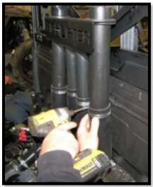
61. Find the rear differential vent hose and remove the 90 degree vent line fitting on the end.
