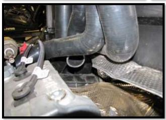
49. Loosely insert two **SK-P-223** (2 x 13 ½" pipes) into the riser plate. You need to align them up so you can determine where to trim the plastic lip on the back of the cab in the next step.
