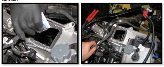
23. Slide the factory metal mount bracket onto the new **75N** clutch outlet duct. While installing, be careful not to pull the sides of the duct in. **This is necessary to prevent it from having an improper seal.** Once fastened, you will need to reach into the housing with your fingers and check for leaks or pulling of the edges.
