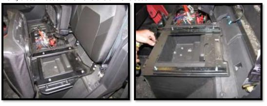
4. Under the passenger seat, lift and remove the storage box. Remove the battery and the battery support bracket. This will give you access to the factory intake hoses.
