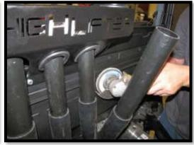
51. Slide the risers back into the riser plate. Then loosely attach the two **43R** riser caps to the top of the risers so that they sit flush to the riser plate. Do not fasten the hoses yet with clamps, you may need to make more adjustments in the following steps.
