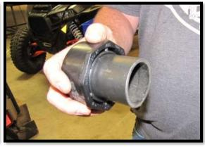
38. Insert the bushing adapter into the factory clutch intake hose and tighten the factory hose clamp.
