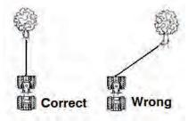
Short pulls from an angle can be used to straighten the vehicle. Long pulls should be done with the wire rope at a 90° angle to the winch/vehicle.
