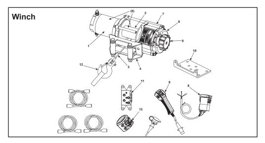
**Motor (1):** 1.7 HP 12V DC motor provides power to the planetary gear mechanism.
