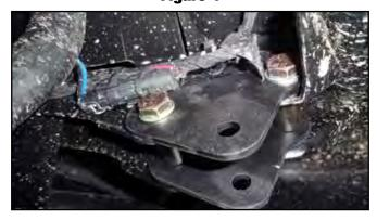
Install a 3/8" washer and 10mm nut to the back side of the two bolts. 8.
