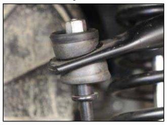
Note: Getting the nuts started again on the sway bar links can be difficult. The sway bar may need to be pushed down to compress the lower bushing so that the nut can be tightened. If this is still not enough to get the nuts started, you can also put a strap around the sway bar (just inside of the bushing assembly) and around the lower a-arm. Tightening down on this will compress the bushing assembly a little more and expose more threads.
