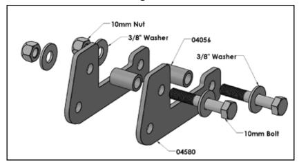
19. Slide the rear brackets inside the factory shock mounts followed by a spacer sleeve. Use a 10mm bolt and 3/8" washer to hold the rear bracket in place.
