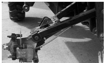
4. Remove the bushings and sleeves from the stock control arms. You will need to reuse these in the new lower arched a-arm kit.
