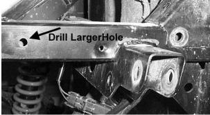
7. Attach the new shock relocation bracket to the top shock mount. You will be moving the top of the shock forward.
