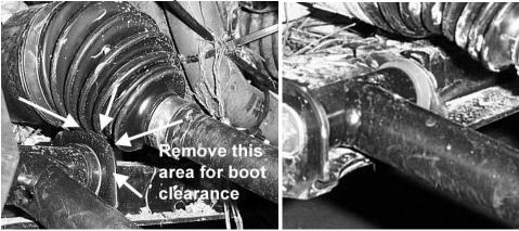
16. Use the factory nuts and bolts to connect the new A-arms to the UTV. Each arm is labeled relative to its location on the UTV. The location is determined from the seated position. You will have left and right upper A-arms and left and right lower A-arms.
