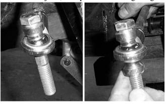
24. Insert the bolt into the knuckle assembly. Place the ½" flat washer and ½" lock nut onto the bolt and tighten.
