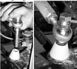
22. Place the ½" washer and ½" lock nut on the bolt and torque tight.
