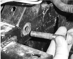
6. Using the stock hole in the frame a pilot hole drill a larger hole using a 13/32 drill bit.
