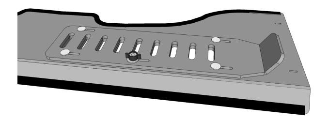
5. Now place the windshield inside the frame of the General. Take the Metal brackets and bolt them to the windshield from the inside using the supplied 1" bolts washer and thumbnut as shown in the picture below.
