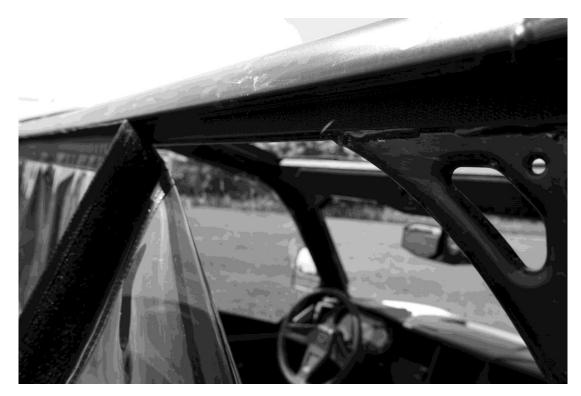
3. After the adhesive Velcro strips have been installed along the top and down the sides you can now place your rear window in the frame. Lastly mark where the bottom of the rear window sits on the vehicle and place the 48" adhesive strip flat on the vehicle so the bottom of the rear window pulls into the cab and attaches downwards.
