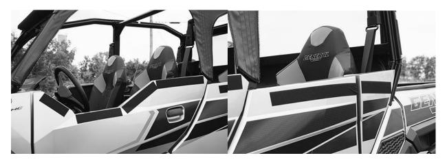
9. Begin the Rear Window by installing the 51" adhesive strip along the top of the rear window frame. The adhesive should be on both sides of the channel. Then install the two 20" strips down the sides. Clean the areas of any dirt or grease before applying adhesive strips.
