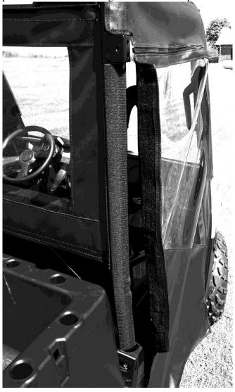
9. Now move to the front bottom edge of the door frame and install the 1" adhesive strip as shown in the photo below.
