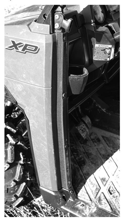
10. Now move to the bottom edge of the door frame and install the snaps as shown in the photos on the next page.
