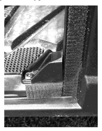
8. After all the Velcro is in place take the door and place it on the vehicle. the following series of photos show how it should look after being installed.
