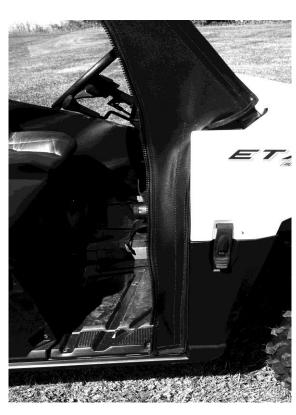
9. Lastly install the snap studs into the plastic for the bottom rear portion of the door. It works best to put the screw studs into the snap sockets on the door first. Then one by one pull the door in place and push the screw into the plastic making sure to put enough pressure to leave a mark. Then remove the screw stud from the door and install it where the mark was left behind at. The following pictures show what it looks like.
