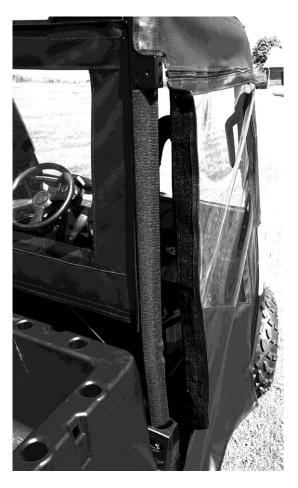
7. Now move to the front bottom edge of the door frame and install the 30" adhesive 1" wide Velcro strip. At the bottom place the 3" strip perpendicular as shown in the photos on the next page.
