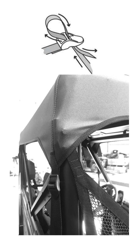
4. Moving to the front of the vehicle you will now need to raise the hood to reveal frame. Again take the looped end of one of the straps and run it around the frame just below the hood line. Then run the other end of the strap through the loop and pull it tight. Photo below shows how it should look.
