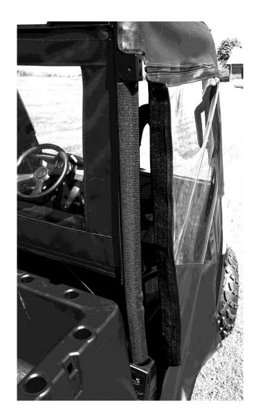
9. Now move to the front bottom edge of the door frame and install the 30" adhesive 1" wide Velcro strip. At the bottom place the 3" strip perpendicular as shown in the photos on the next page.
