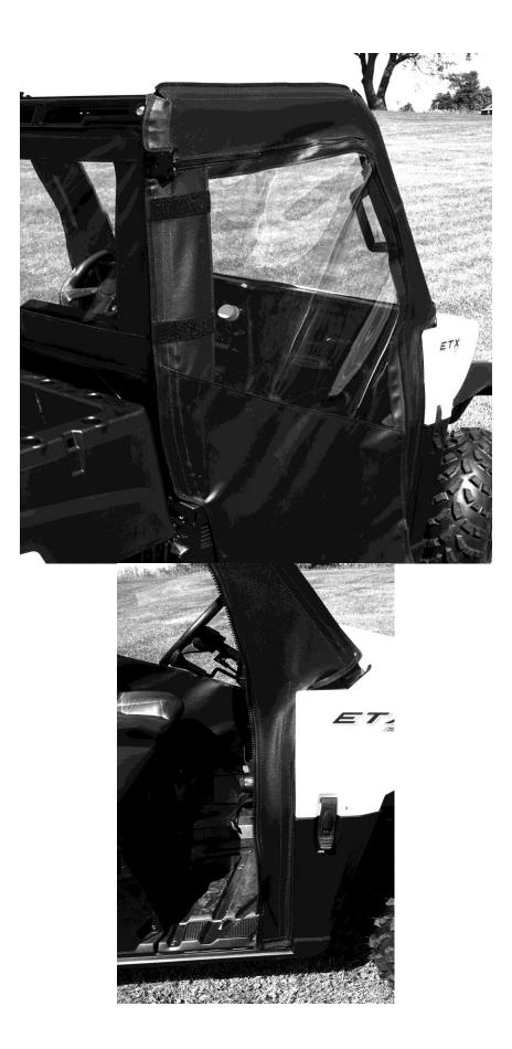
11. Lastly install the snap studs into the plastic for the bottom rear portion of thee door. It works best to put the screw studs into the snap sockets on the door first. Then one by one pull the door in place and push the screw into the plastic making sure to put enough pressure to leave a mark. Then remove the screw stud from the door and install it where the mark was left behind at. The following pictures show what it looks like.
