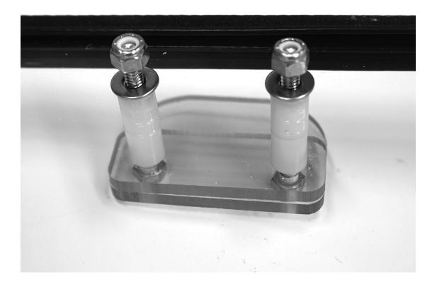
8. Now that the gasket and bottom brackets are in place it's time to place the Rear Window in place on the vehicle. The brackets are designed to hold the window in place along the bottom of the frame in behind the seats as shown in the photo below.
