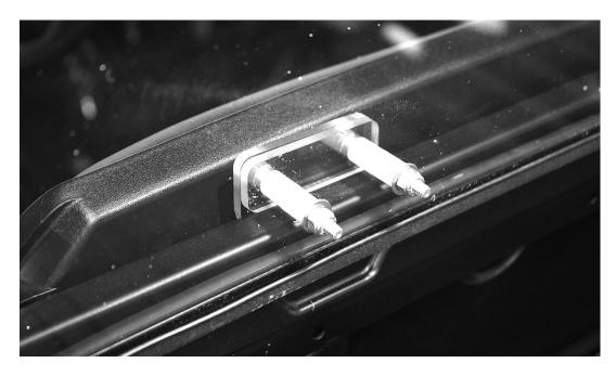
9. Once the Rear Window is in place and properly centered on the vehicle the final step is to install the brackets across the top of the window to secure it in place. This is done the same as the bottom brackets except you use just one spacer per bolt instead of two. See photo below
