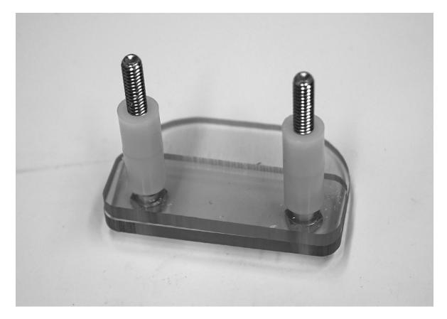
6. Now take the two plates and spacers and insert them into the holes along the bottom so that the plates are on the inside or the gasket side of the windshield. See photo below.
