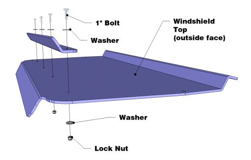
• Now you are ready to place the windshield on the Ranger and attach to the outside of the roll cage. NOTE: THE BEND AT THE TOP OF THE WINDSHIELD SHOULD GO BELOW THE TOP TUBE. The diagram on the next page shows the proper placement for the hardware. Install the clamps as shown for the top two slots in the windshield only. Use the 1" bolts for this application.
