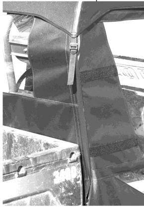
**C.** Diagram below shows how to use ladder buckle.
