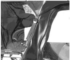
**b.** Next take the other two long straps and wrap them around the roll cage in the rear just under door and rear window at the very bottom of the roll cage. Pull the strap up and connect to the buckle at the rear of the top.
