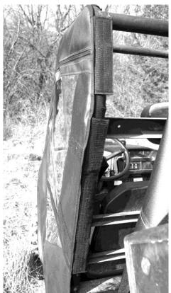
3. Once all the Velcro is in place the last thing to do is install the screw snap studs. NOTE: The best way to install the snap studs is to put them in the sockets in the door first. Then push them into the plastic to make an mark. Then pull the screw stud out and screw it into the plastic where the mark was made. See Photos Below.
