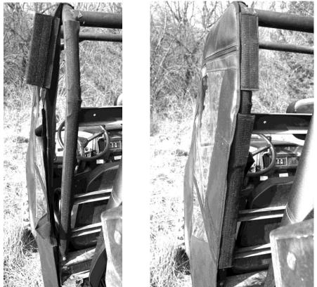
3. Once all the Velcro is in place the last thing to do is install the screw snap studs. NOTE: The best way to install the snap studs is to put them in the sockets in the door first. Then push them into the plastic to make an mark. Then pull the screw stud out and screw it into the plastic where the mark was made. See Photos Below.
