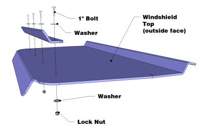
• Now you are ready to place the windshield on the Ranger and attach to the roll cage. NOTE: THE BEND AT THE TOP OF THE WINDSHIELD SHOULD GO BELOW THE TOP TUBE. The diagram on the next page shows the proper placement for the hardware. Install the clamps as shown for the top two slots in the windshield only. Use the 1" bolts for this application.
