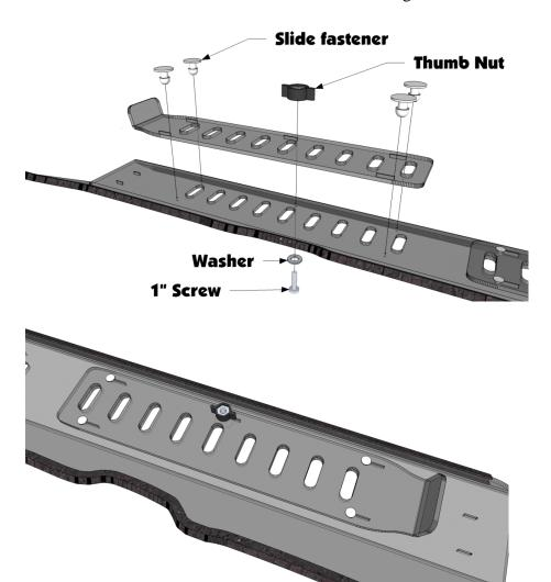
• Next take the bent Lexan brace and install it on the windshield. Please see diagram Below.
