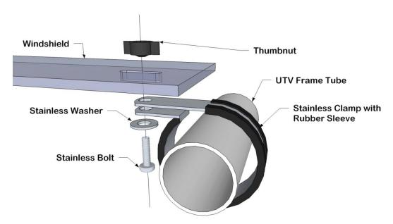
• Now Place the two halves onto the frame as shown below.
