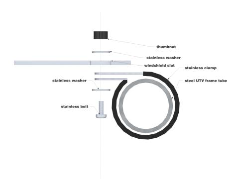
• Now install the clamp for the slot right above the hinge. You will use the 1 ¼" bolts for this. Below is the diagram showing how this is installed. You will have some of the bolt sticking out towards the front of the vehicle. This is to hold the bottom section of the windshield when it is in the raised position. You will use the same thumb nut for the raised and lowered positions.
