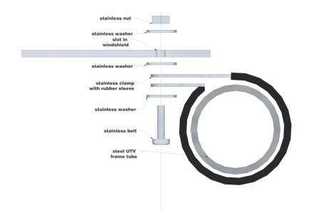
• Finally install a clamp around the tube blow the hinge as shown below. You will use the 1 1/4" bolts here. This clamp holds the bottom of the windshield down.
