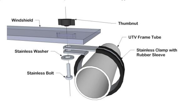
6. Now Place the two halves onto the frame as shown below.
