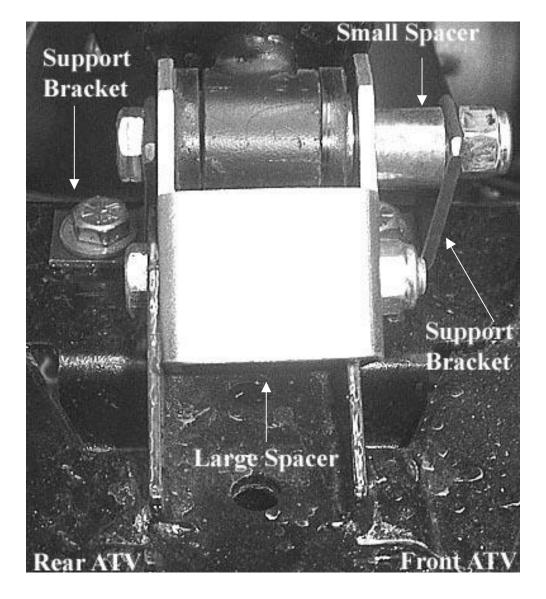
7) Connect the rear support bracket to the frame using the ½ x ¾ hex bolts, ½ washers, and ½ locking nuts. Use the holes already in the frame from the factory to connect to the frame.
