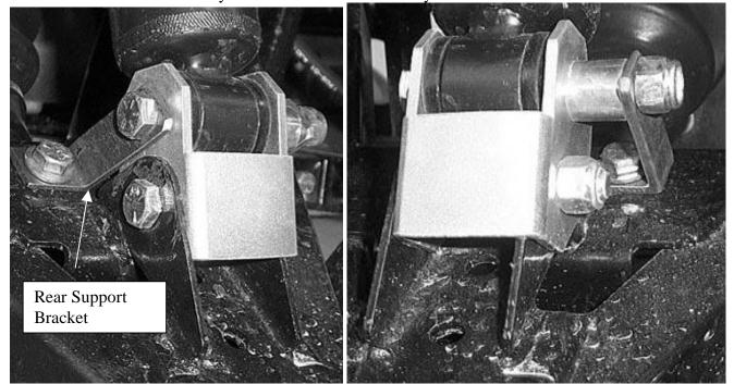
8) Remove factory the torsion bar bracket and install new bracket on the torsion bar and axle using the factory bolts. This bracket is just like the factory bracket except it is slightly larger.
