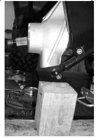
11) Lower the jack, this will place weight on the end of the strut that is connected to the control arm. This
