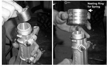
7) Slide the strut cartridge back into the socket.
