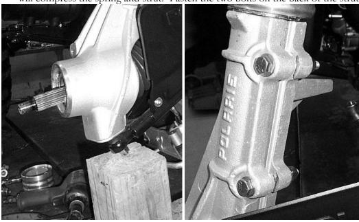
12) Reconnect the tie rod, hub, and brake assembly. Reconnect the hub assembly using the new castle nut provided in the kit. Leave off the factory conical washer. **Make sure to secure it with cotter pin.**
