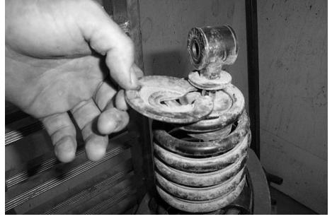
5) Next remove the spring and place the rear spring spacer onto the shock.
