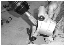
29. Connect the upper arm to the hub assembly using the factory hardware.
