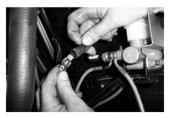
26. Reconnect it to the caliper using the factory hardware.
