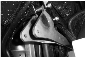
33. Use two 10mm x 35mm bolts to secure the short front lift brackets to the long front lift bracket.
