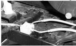
14. Disconnect the brake lines from the junction fitting. Connect the new extension to the brake lines now.
