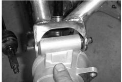
30. Connect the lower arm to the hub assembly using the factory hardware.
