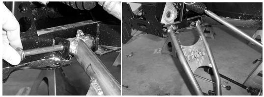
39. When you have the lower arm in place, insert the new front axles into the differential.
