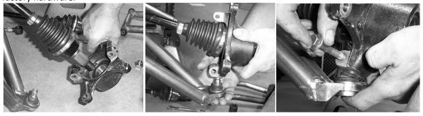
41. Next, connect the upper control arm to the frame and then to the hub assembly. Use the factory hardware.
