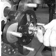
5. Remove the brake rotor.
