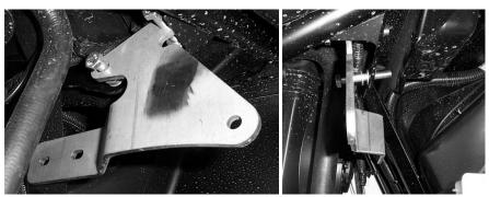
32. Now insert a spacer on each of the bolts and the other front long lift bracket to the inside of the shock mount tab. Loosely fasten it with two 10mm lock nuts.
