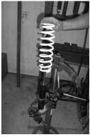
22. Next place the spring spacer onto the shock.
