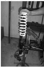
20. Next place the spring spacer onto the shock.
