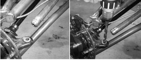
52. Provided in the kit is a heim joint that will connect to the tie rod. Place on the heim joint a jam nut. We recommend that you run the jam nut all the way down the threads.
