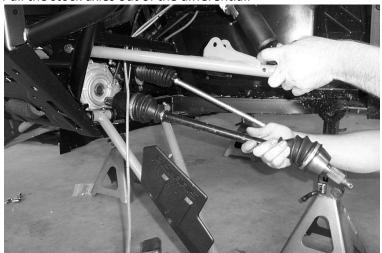
8. Disconnect the tie rod ends from the tie rods.
