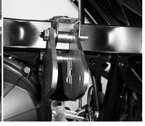
37. Connect the top of the shock to the lift brackets using one 10x65mm hex bolt and 10mm lock nut.
