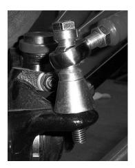
56. Place the  $\frac{1}{2}$ " washer and  $\frac{1}{2}$ " lock nut on the bolt and torque tight.
