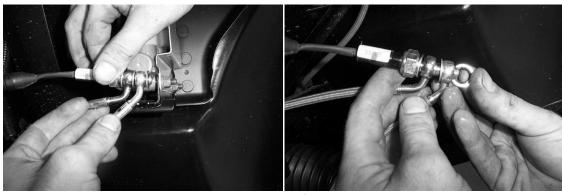
25. Now install the new longer line on the right side of the UTV. Connect it to the master cylinder using the factory hardware.
