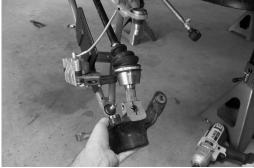
7. Pull the stock axles out of the differential.
