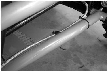
42. In the kit, there is a P-clamp, 6mm x 20mm bolt, 6mm washer, and 6mm lock nut. You will fasten the brake line to the lower control arm using the P-clamp and hardware.
