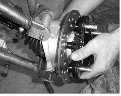
32. Fasten the rotor using the axle washer, castle nut, and cotter pin provided in the kit.
