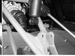
10. Unclip the brake lines from the control arms. Tie the calipers up out of the way.
