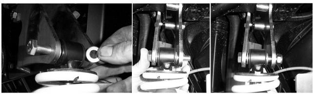
47. Connect the lower portion of the shock to the new control arm using the factory hardware.
