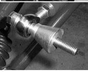
55. Insert the new  $\frac{1}{2}$ " x 4-1/2" hex bolt. Slide the bolt through the alignment bushing, large cone then the heim joint and then through another alignment bushing. Insert the bolt through the knuckle assembly.
