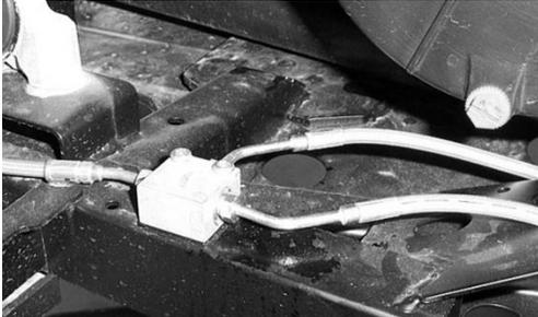
14. Disconnect the brake lines from the junction fitting. Connect the new extension to the brake lines at this time.
