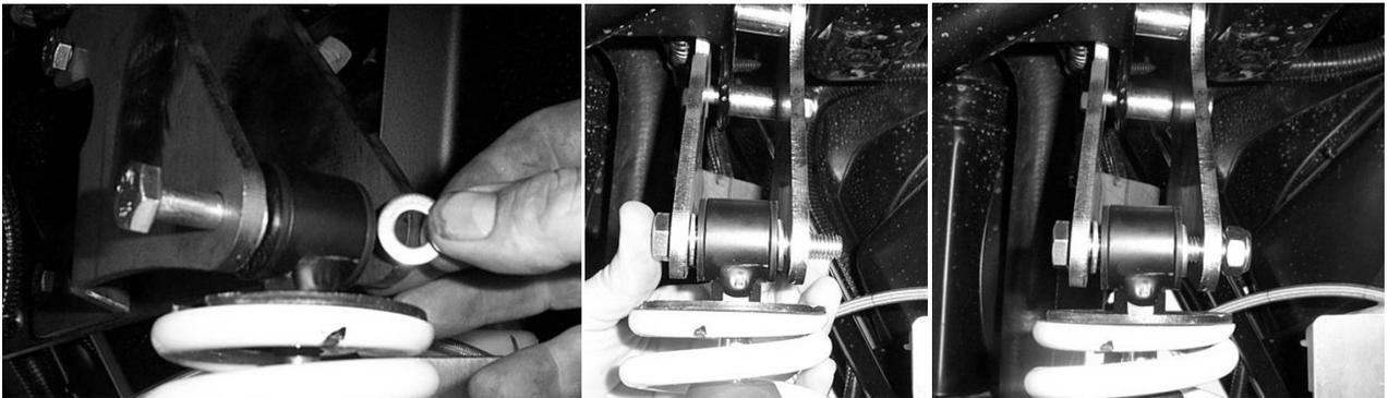
49. Connect the lower portion of the shock to the new control arm using the factory hardware.
