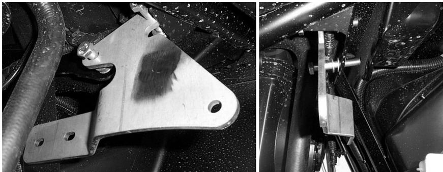
31. Now insert a spacer on each of the bolts and the other front long lift bracket to the inside of the shock mount tab. Loosely fasten it with two 10mm lock nuts.
