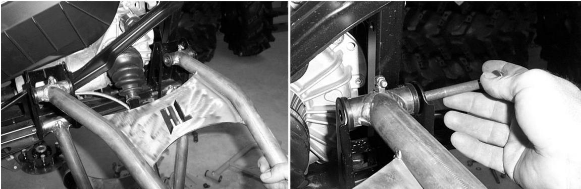
28. Now, slide the hub assembly over the axle end.
