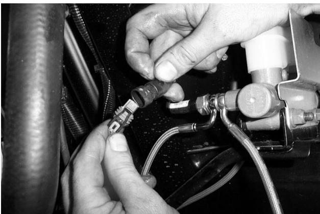
26. Reconnect it to the caliper using the factory hardware.
