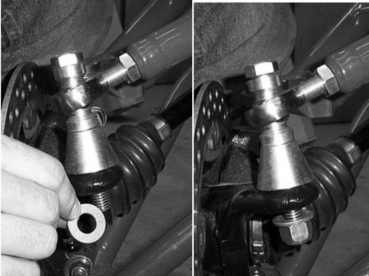
57. When you have completed the tie rod installation on both sides you will need to adjust to achieve the proper alignment.
