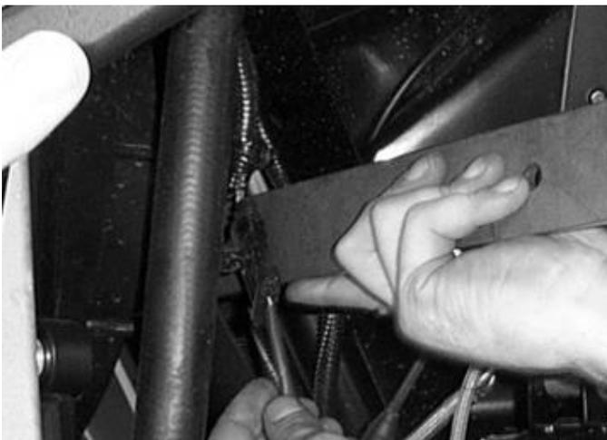
30. Depending on which side you are working on you will place either a left lift bracket or right lift bracket to the outside of the front shock mount. It needs to be on the side that faces the front of the UTV. Connect the bracket using two 10x65mm hex bolts and four 10mm flat washers. Insert the two bolts through the bracket, then place two washers on each bolt. Insert the bolts through the shock mount tabs.
