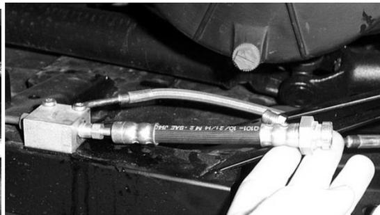
15. Reconnect the new brake extension lines to the brake line junction. You may need to do some re-routing at a later point to ensure that there is no pinching of the brake lines.
