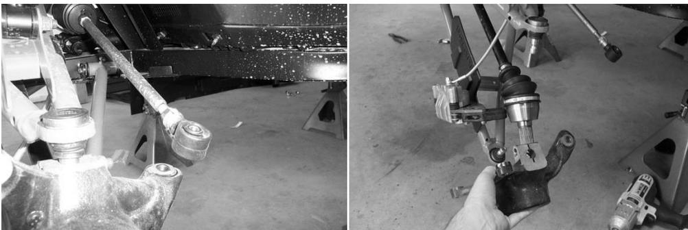
7. Pull the stock axles out of the differential.
