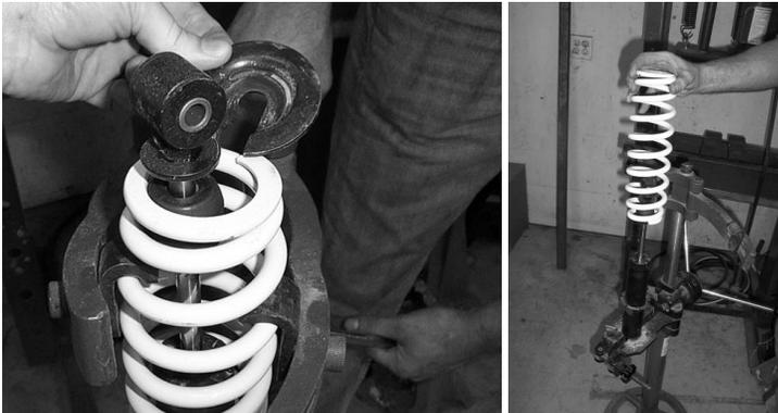
22. Next place the spring spacer onto the shock.
