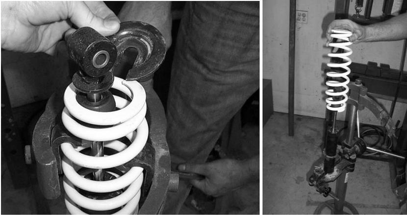
20. Next place the spring spacer onto the shock.
