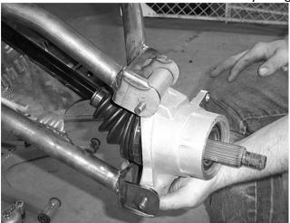
31. Place the rotor onto the hub and axle assembly.
