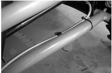
42. In the kit there is a P-clamp, 6mm x 20mm bolt, 6mm washer, and 6mm lock nut. You will fasten the brake line to the lower control arm using the P-clamp and hardware.
