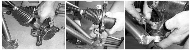
44. Next, connect the upper control arm to the frame and then to the hub assembly. Use the factory hardware.
