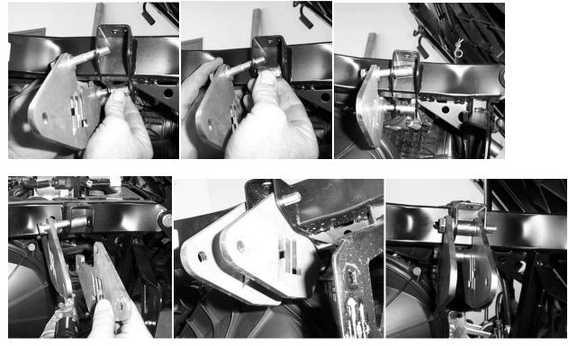
37. Connect the top of the shock to the lift brackets using one 10x65mm hex bolt and 10mm lock nut.
