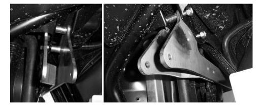
32. Use two 10mm x 35mm bolts to secure the short front lift brackets to the long front lift bracket.
