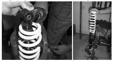
22. Next place the spring spacer onto the shock.
