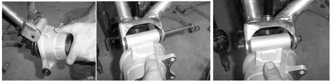
30. Connect the lower arm to the hub assembly using the factory hardware.
