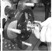
5. Remove the brake rotor.
