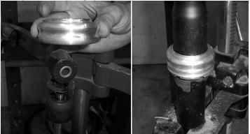
23. Place spring back on the shock, compress it, and then reinstall the retaining clip.
