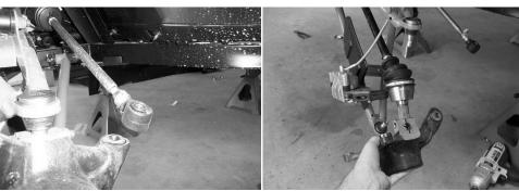
7. Pull the stock axles out of the differential.
