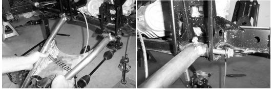
26. Next install the rear axles into the differential.
