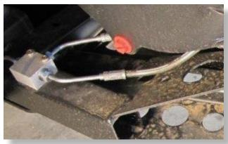
Install the new 63" REAR RIGHT brake line to the block, then the 55" REAR LEFT line.
