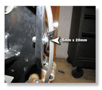
Secure the line to the portal backing plate using a p-clamp and the 5mm x 20mm bolt, 5mm washer, and 5mm lock nut.
