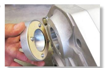
Remove the  $1/4-20 \times 3/4$ " screws & cap/gasket from the lid of the portal box.
