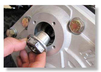
Apply LOCTITE (BLUE) to the supplied M18 axle nut with shoulder PGLC-AXNUT-4 and torque onto the drive shaft axle. (30mm) [20 ft lbs]
