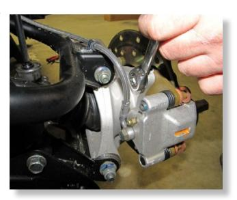
**Remove the brake caliper mounting bolts** from the hub assembly. **(15mm) KEEP FACTORY HARDWARE.**
