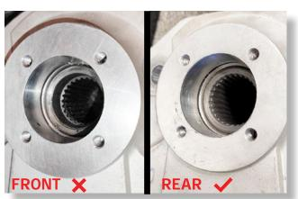
NOTE: On the REAR portal boxes, the drive gear is reversed, and the splines should be to the outside edge to accommodate the longer rear drive shaft splines.
