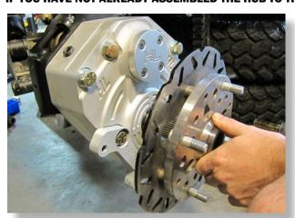
**Apply waterproof grease to the spindle splines** and slide the brake rotor assembly onto the spindle shaft.
