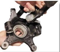
Disconnect the **Lower ball joint** by removing the **bolt** at the knuckle. (15mm)
