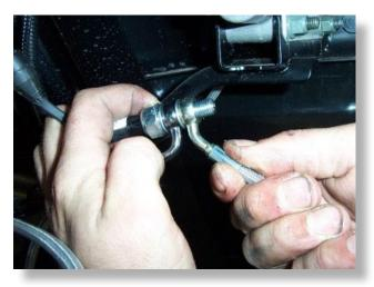
Install the new 50" FRONT LEFT brake line to the banjo bolt. Run the line back through the frame and to the LEFT (DR) side hub.
