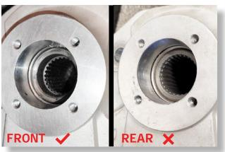
NOTE: On the FRONT portal boxes, the drive gear splines should be recessed to accommodate the shorter front drive shaft splines.
