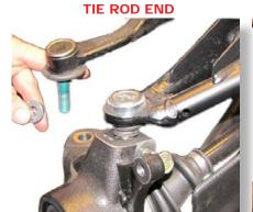
Disconnect the tie rod from the knuckle. (18mm)
