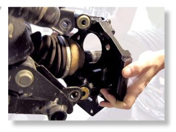
Place the backing plate into position on the control arms and guide the drive shaft through.
