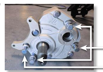
Insert the washers and bolts below through the remaining (4) holes in the rear portal box.
