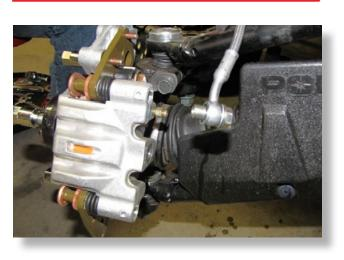
Disconnect the **stock brake line from the caliper**, if you have not done so already.
