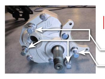
Insert the washers and bolts below through the remaining (4) holes in the front portal box.
