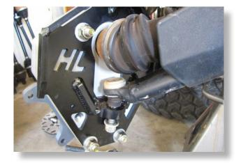
Loosely fasten all (4) bolts with 1/2" flat washers and 1/2" lock nuts. Ensure parts fit correctly then torque. (3/4) [105 ft lbs]
