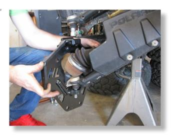
Insert the lower ball joint into the lower mount bracket on the backing plate.
