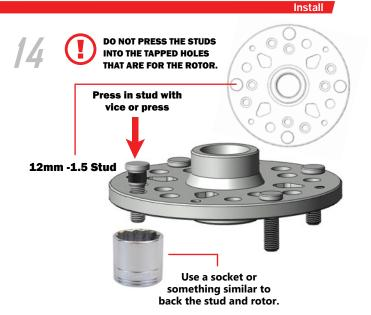
ROTOR ASSEMBLY Install
