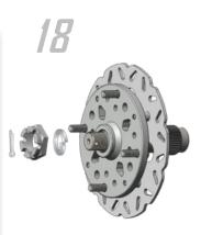
Slide on the 30mm lock washer, 30mm castle nut. (46mm) [Min 120 ft lbs]
