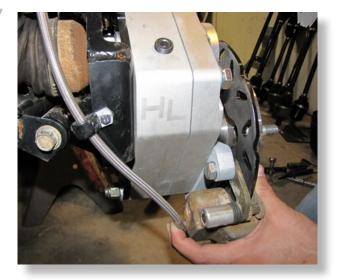
Reattach the brake line to the caliper.
