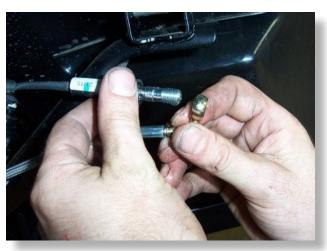
Install the **58**" **FRONT RIGHT brake line** to the banjo bolt. Run the line back through the frame and to the **RIGHT (PA) side hub.**
