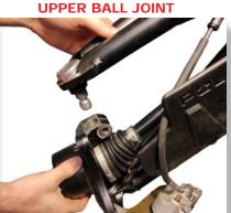
Disconnect the **Upper ball joint** by removing the **bolt** at the knuckle. (**15mm**)
