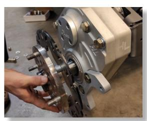
**Apply waterproof grease** to the spindle splines and slide the brake rotor onto the spindle shaft.
