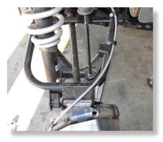
NOTE: ENSURE THAT THERE IS NO BINDING, PINCHING, OR INTERFERENCE WITH MOVING PARTS AND THE NEW BRAKE LINES. BLEEDING BRAKES \_\_\_\_\_ Brake Lines
