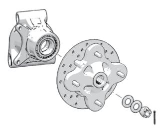
Remove the cotter pin and castle nut (27mm) on the rear axles, then remove the brake rotor assembly.
