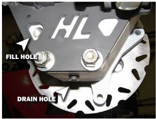
**Use SAE 80W-90 oil.** This gear lubricant is designed for gears operating under severe temperature and load conditions. **SAE 80W-90** viscosity grade offers extended performance.
