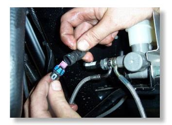
Fasten banjo bolt to master cylinder. Torque (12mm) [50 ft lbs)
