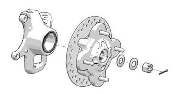
Remove the cotter pin, axle nut, and washers from the hub assembly, then remove the hub. (27mm)
