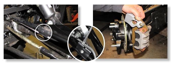
Disconnect **brake lines** from arms and frame. Remove the **brake caliper mounting** bolts (15mm) Remove the **front mud scraper (8mm). KEEP ALL FACTORY HARDWARE.**
