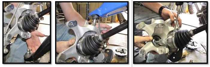
NOTE: If you are experiencing difficulty removing the upper ball joint unbolt the lower shock and sway bar.
