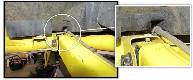
e. Disconnect and remove all <u>rear</u> brake lines from the master cylinder. Start by disconnecting the rear supply line from the master cylinder under the steering wheel. **Have area prepared for brake fluid clean up**.
