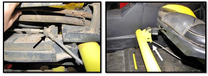
c. Drill out the rivets securing the factory p-clamps to the trailing arms.
