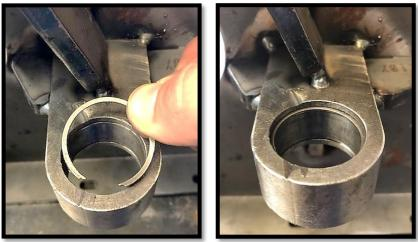
h. Find a 13/16 socket or pipe to press the joints in. We recommend applying a small amount of grease to the joint, then place it <u>straight</u> into the bracket. Use a press or vise to press it in until it stops at the retaining ring.
