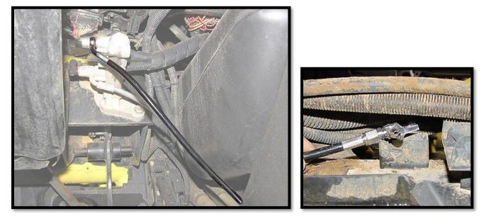
g. Route the new 96" rear left (driver side) and 96" rear right (pass. side) brake lines from the t-block and back down to the calipers. <u>Make sure the orientation is correct and secure the new brake lines to the t-block</u>. And then attach the brake line to the caliper.
