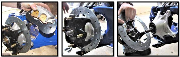
d. Remove the nuts that attach the rear knuckle to the radius bars. (18mm) <u>Only pull the bolts out far enough</u> so that the knuckle can be released. This way you don't have to disconnect the radius bars. Then remove the knuckle.
