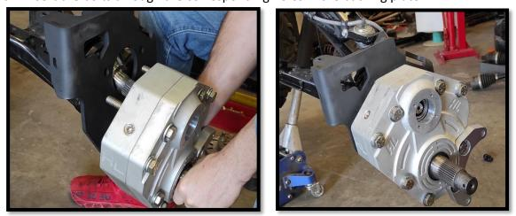
**Loosely fasten all (4)** bolts with **1/2**" **flat washers and 1/2**" **lock nuts. Ensure parts fit correctly then torque.** (3/4) [105 ft lbs]
