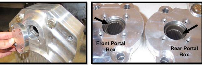
c. Find the caliper mounting bracket **129Z** and place it in the corresponding fitted <u>FRONT</u> section of the portal box.
