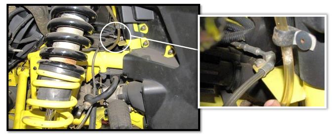
d. Disconnect the front supply line from the master cylinder under the steering wheel. Have area prepared for brake fluid clean up.
