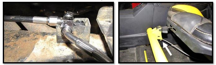
j. Slide a **p-clamp (WL-CLAMP-12)** over the brake line. Secure it to the rear backing plate using a **5mm x 20mm bolt** through the clamp and backing plate, followed by a **5mm washer** and **5mm lock nut.**
