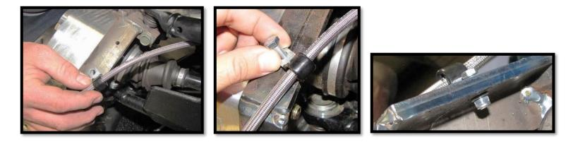
k. Secure any remaining brake line slack by using **zip ties**. <u>Make sure there's no binding in the lines once</u> <u>they're secured, even at full turn.</u>
