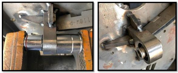
i. Once the second retaining ring groove is visible, you can then re-install the boot. Use a flat head to press it back in and take care not to damage it. Then place and snap in the second **retaining ring 115M**.
