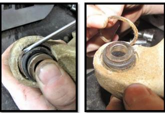
c. On the other side of the joint, the knuckle has a built in stop. Find a socket or tool to fit the inner diameter of the stop. Then use a press or a vise to remove the joints.
