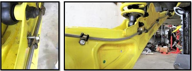
i. Fasten the new t-block to the factory location using the factory hardware. **Do not over-torque**. And then secure the brake lines to the seat frames using the factory nuts.
