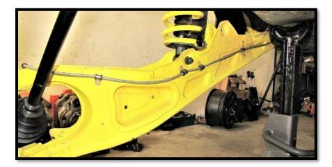
d. There's one rivet that isn't easily accessible. You can either remove the seats and drill through the plastic to remove them. Or what we recommend, you can simply cut the brake lines near the p-clamp (Have area prepared for brake fluid clean up). The factory lines and <u>this p-clamp</u> will not be re-used.
