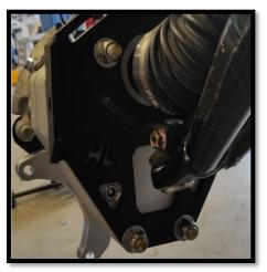
d. Install the tie rod end into the backing plate tie rod mount bracket. Fasten the tie rod end with the factory hardware. (18mm) [90 ft lbs]
