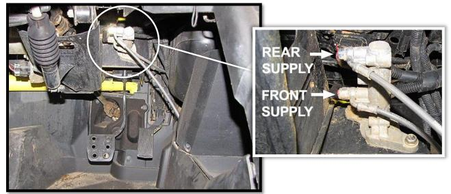
f. Install the new **28**" rear supply brake line to the master cylinder. Then install the new **t-block**. Do not secure the t-block yet to factory location.
