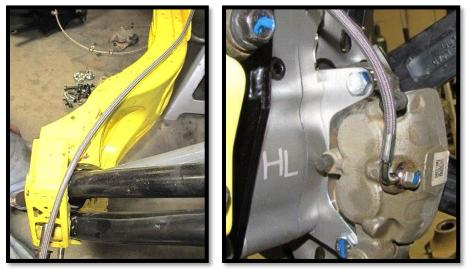
h. Next, pull any extra slack out from the caliper to under the seat. Then re-use your factory p-clamps to secure the new brake lines to the trailing arms. Insert a 6mm x 12mm screw through each clamp and fasten them. Do not over-torque!
