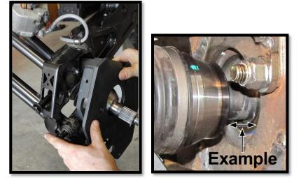
e. Insert all radius bar hardware into the backing plate and fasten them. (15mm)
