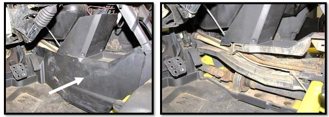
b. Disconnect the factory t-fitting from its fitted section. And then remove the nuts securing the factory brake lines to the bottom of the seat frames.
