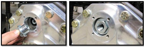
c. Align the portal box lid cap & gasket. Use the 1/4-20 x 3/4" screws and install to the box. (5/32) [8 ft lbs]
