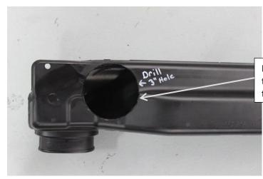
Drill a 3" hole centered on the rear side of clutch intake tube.
