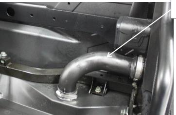
Remove engine air vent. Save clamps.
