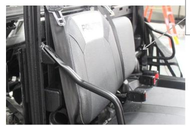
Remove driver side seat/seat back or remove full seat back depending on model. On Crew – rear seat back.
