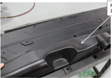
Remove clutch intake tube. 2 #20 torx screws
