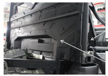
Remove the outer air intakes from the B post - both sides. Save screws and darts. Right side shown with intake removed.
