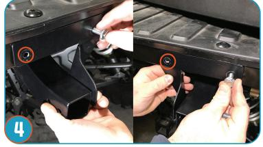
Using the provided hardware secure both brackets to rear of vehicle aligning bolt holes and mounting bars as shown.
