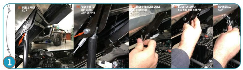
Replace the stock cable located underneath bed of Ranger. (A) Remove top clip (B) Push top pin only enough to remove cable. (C) Loop new cable onto pin. Compress shock by closing the bed. (D) All in one motion raise the bed and push the pin in as this will temporarily relieve pressure on the pin. (E) Re-install clip. Repeat same process for the lower Clip/Pin.
