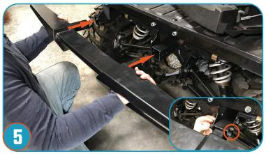
Place bumper on rear of vehicle inserting bumper arms into the mounting bars and secure with provided hardware (4 shorter bolts).
