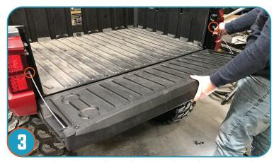
Remove the tailgate by unhooking the cables on each side of the vehicle and pull tailgate up and out and place in bed of your vehicle.
