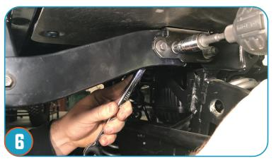
Securely tighten all bolts and nuts applied during the install process.
