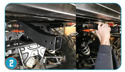
Insert mounting bars to brackets located under bed of Ranger and secure with provided hardware (4-Long Bolts/Nuts). Repeat for other mounting bar.
