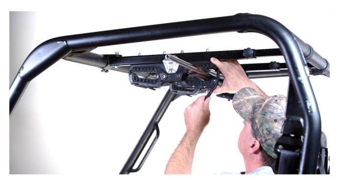
9. Re-Fasten the rubber retention straps, choose whichever hole provides the desired compression and make sure gun is secure before operating the vehicle.
