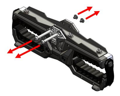
4. Remove the two binding barrel screws from the assembly as shown above and set aside.
