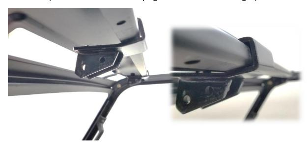
1. Place the profit header bracket B onto the back side of the header panel. Make sure the square portion is fully engaged onto the header panel. Bracket B will be snug on header panel. A rubber mallet may be used to fully engage the bracket onto the header panel.
