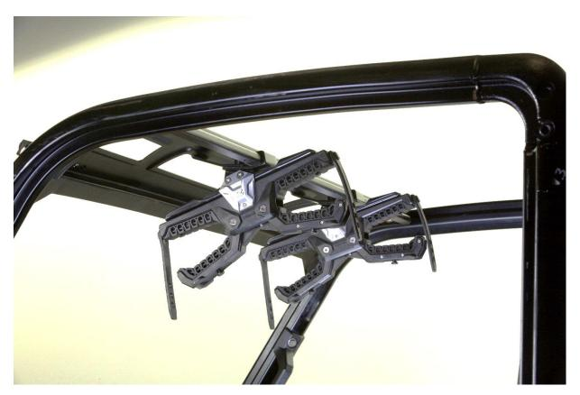
6. Before you tighten the binding barrel screws, test fit your guns into the grips to make sure the spacing is correct. If not, remove the gun grip assembly, loosen the M8X25 bolt, slide the mounts to the desired location and re-install the gun grip assemblies.
