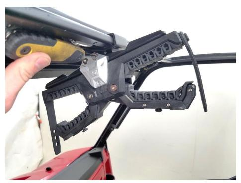
7. Tighten the two binding barrel screws on each grip assembly once you are satisfied with the spacing of the gun.
