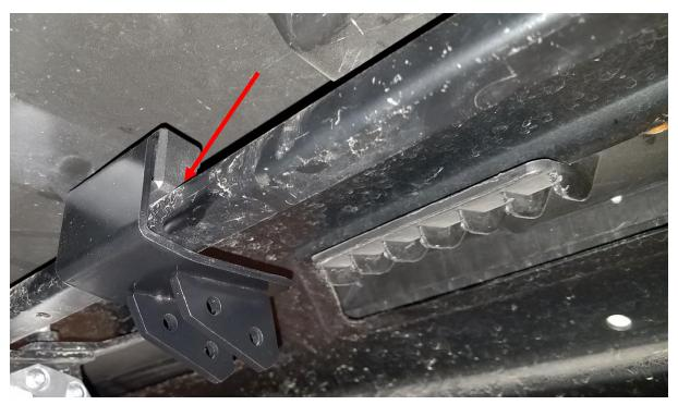
1b. Place the Pro Fit Header bracket B with spacer block E onto the back side of the header panel. Make sure the block portion is fully engaged onto the header panel jog as shown above.
