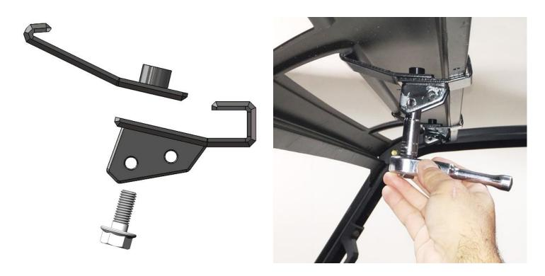
3. Insert the M8x25 flange bolt and tighten. The correct order of the assembly can be seen to the left.
