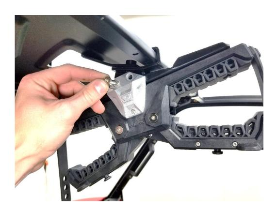
5. Attach the gun grip assembly with the two binding barrel screws to the upper mounts. The two holes will line up with the ears on the bracket.
