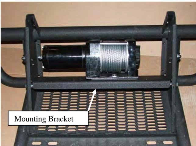
"Figure 3" Install Winch Mounting Plate
