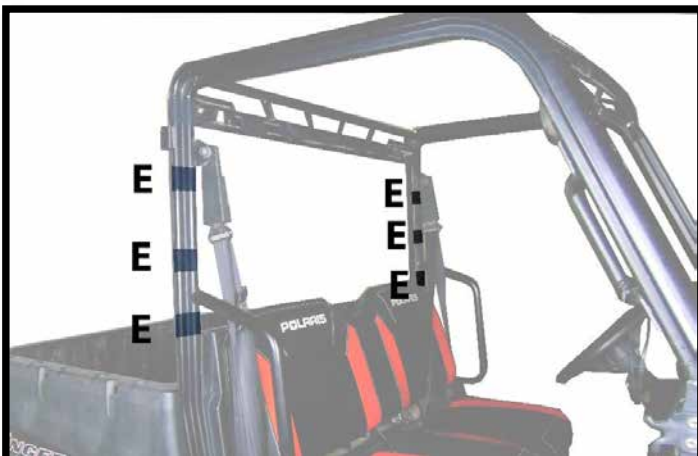
Figure 3: SHOWS PLACEMENT OF 6" VELCRO STRIPS (E)
