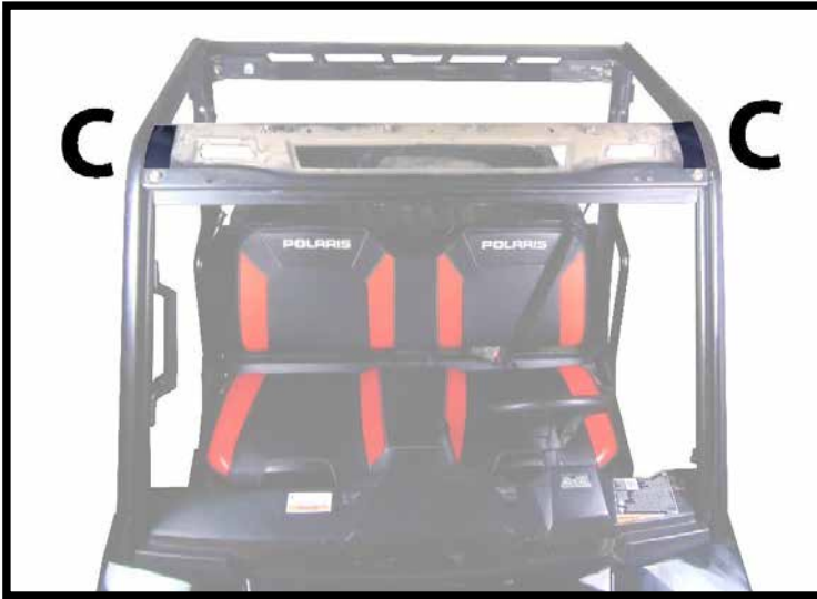
Figure 3: SHOWS PLACEMENT OF 7" VELCRO STRIP (C)
