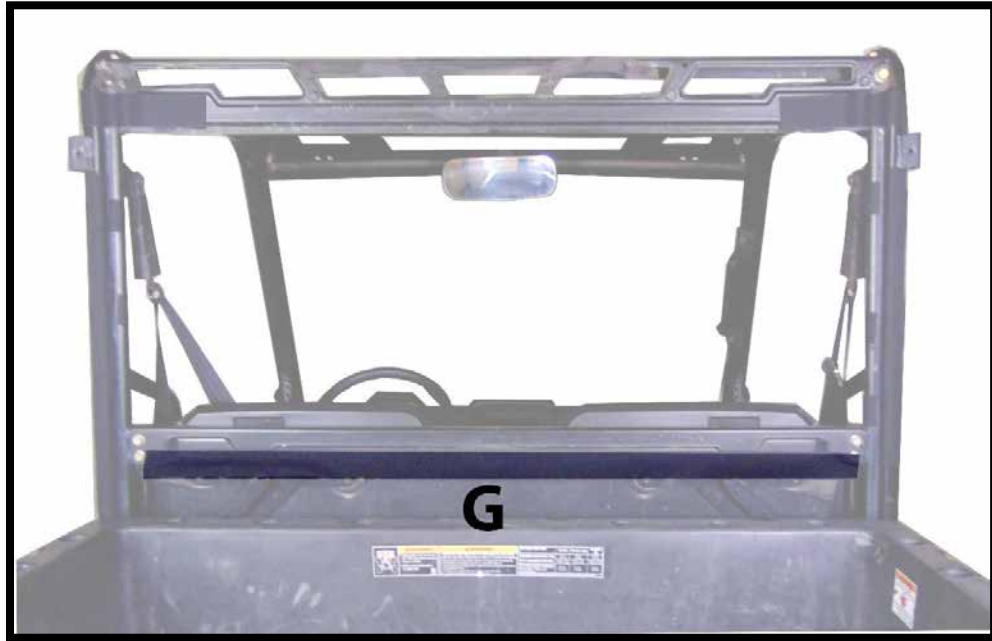
Figure 5: SHOWS PLACEMENT OF 54" VELCRO STRIP (G)
