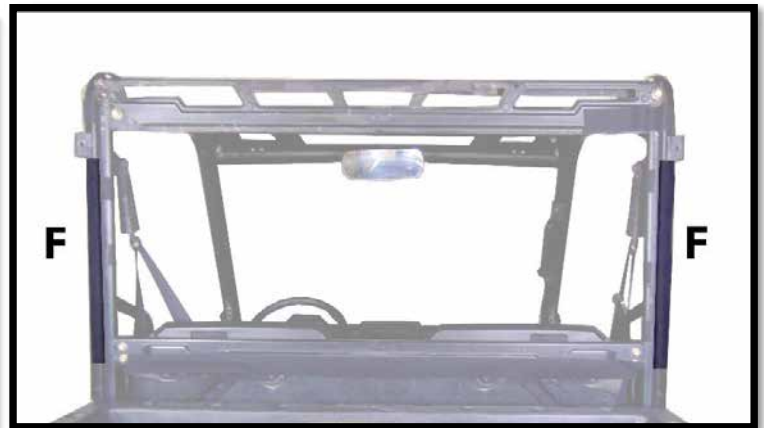
Figure 4: SHOWS PLACEMENT OF 18" VELCRO STRIPS (F).
