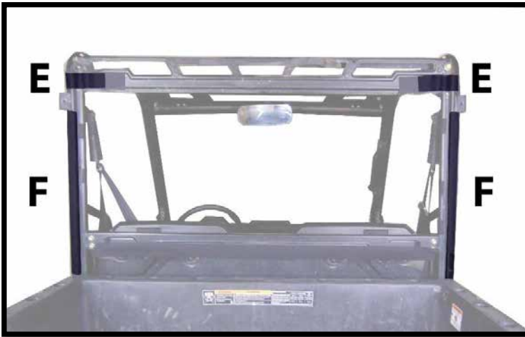
Figure 5: SHOWS PLACEMENT OF 10" AND 22" VELCRO STRIPS (E AND F)
