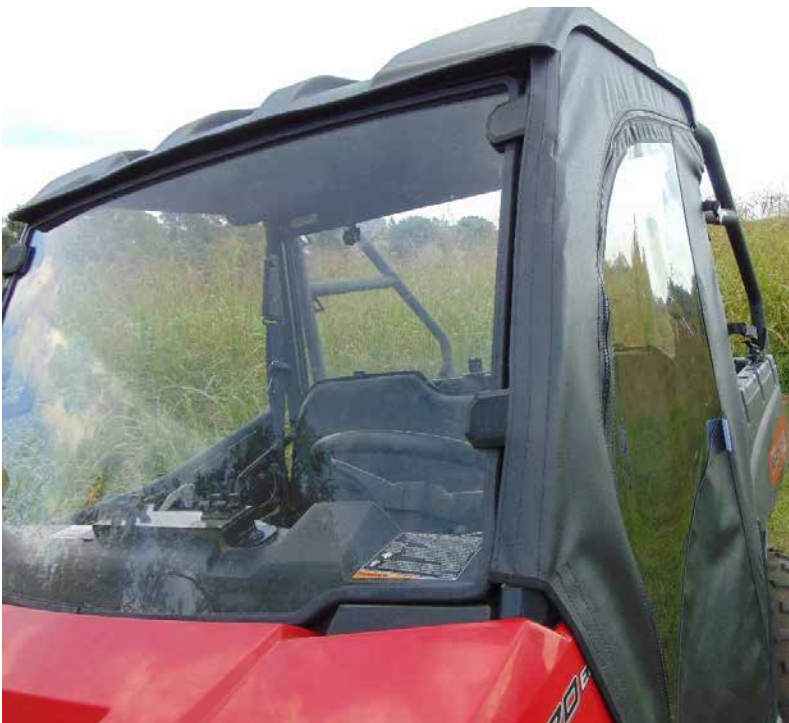
Figure 12: REINSTALL WINDSHIELD AND HARD TOP OVER THE DOOR KITS TABS AND STRAPS.
