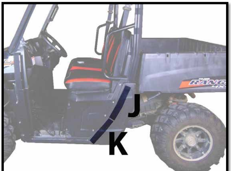
Figure 8: SHOWS PLACEMENT OF 13" VELCRO STRIPS (J AND K).
