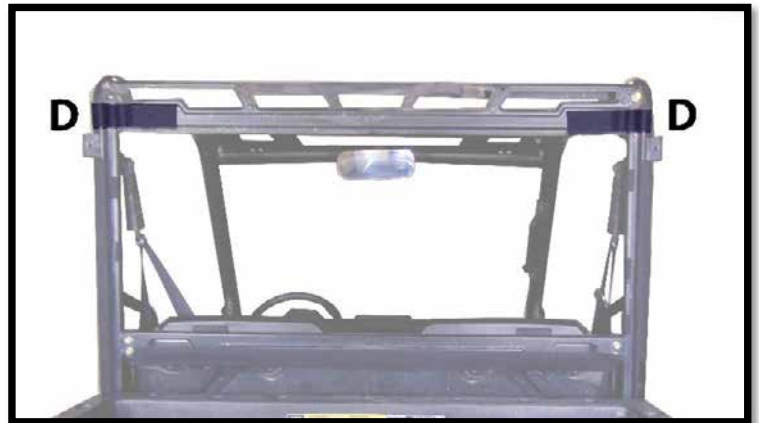
Figure 2: SHOWS PLACEMENT OF 12" VELCRO STRIPS (D).
