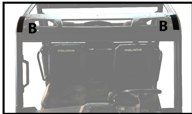
Figure 2: SHOWS PLACEMENT OF 6" VELCRO STRIPS (B)
