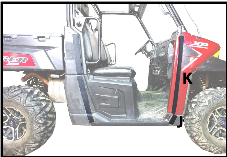
Figure 7: SHOWS PLACEMENT OF 4" AND 29" VELCRO STRIPS (J AND K)
