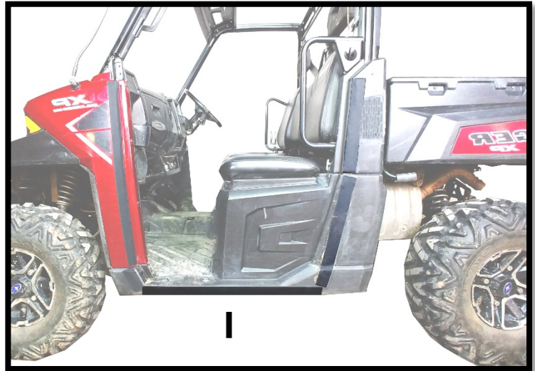
Figure 6: SHOWS PLACEMENT OF 29" VELCRO STRIP (I)
