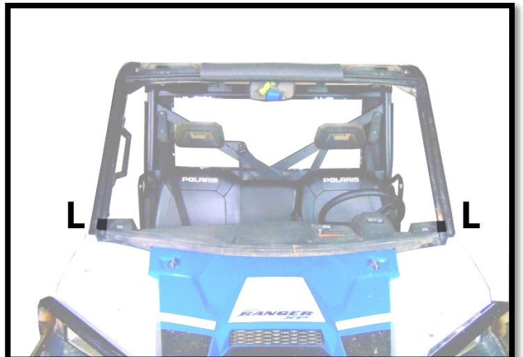
Figure 8: SHOWS PLACEMENT OF 2" VELCRO STRIPS. (L) FOR SMALL STRAP ON THE FRONT OF THE DOOR. PLACE TOWARD THE INTERIOR OF THE CAB NEXT TO DASH.
