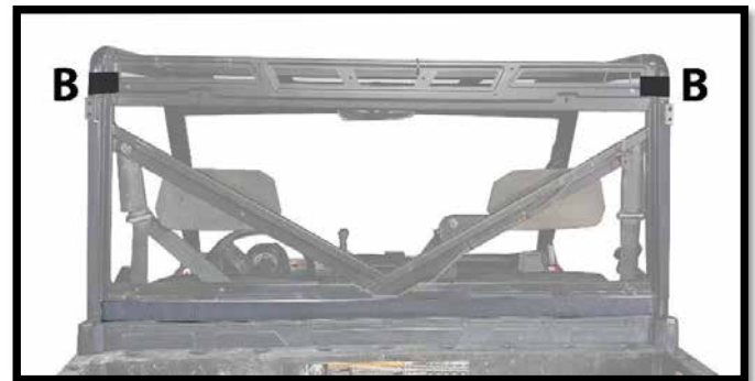
Figure 2: SHOWS PLACEMENT OF 6" VELCRO STRIPS (B).
