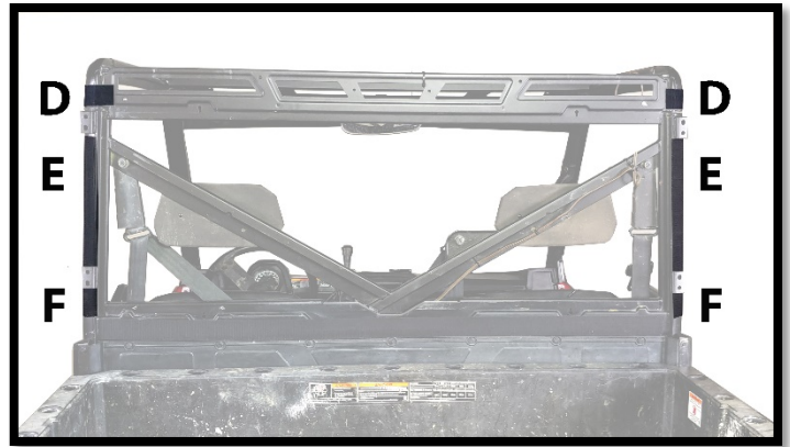
Figure 4: SHOWS PLACEMENT OF 4", 13" AND 3" VELCRO STRIPS (D, E AND F)
