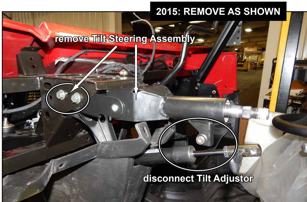
**REMOVAL;** *Keep all components removed from machine.*
