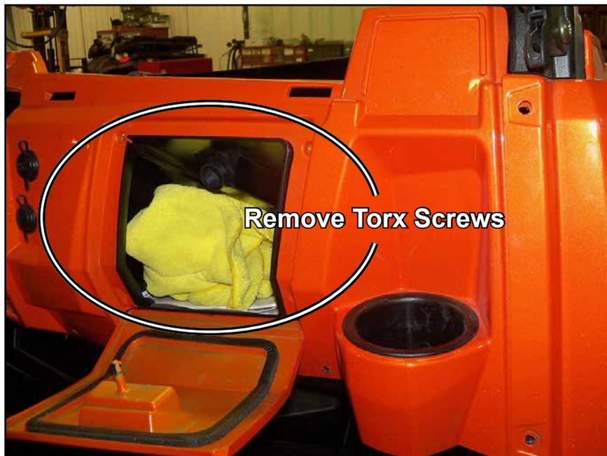
**REMOVAL;** Keep all components removed from machine.
