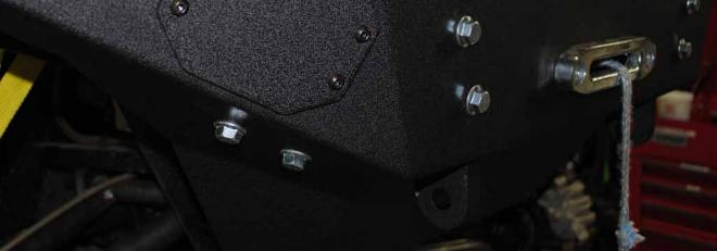
Align Brush Guard to machine and tighten hardware completely.
