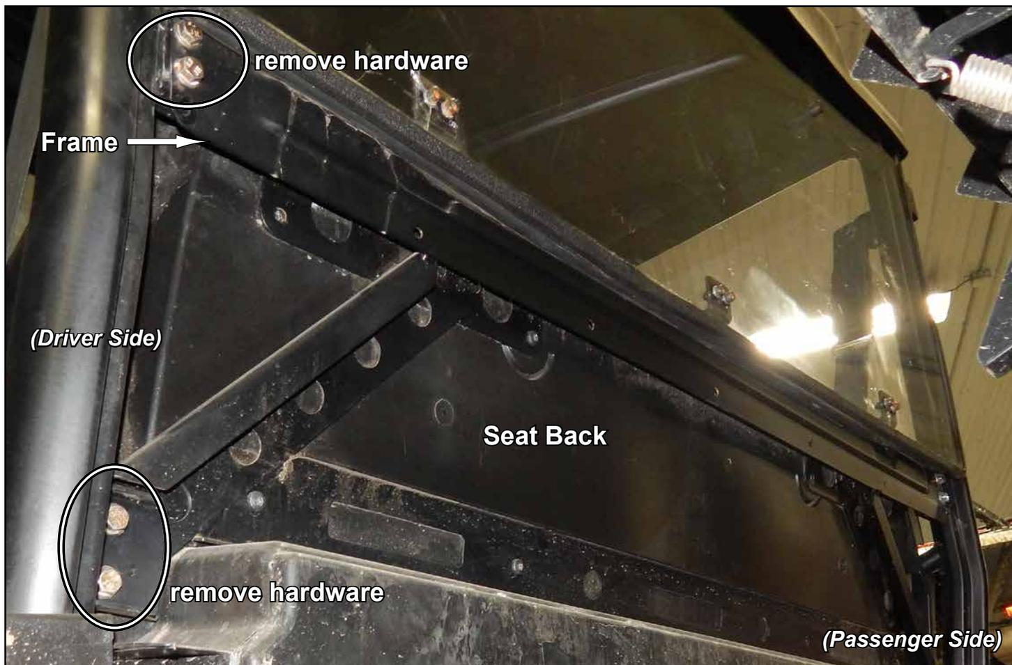
***Do not tighten hardware completely when installing.***
