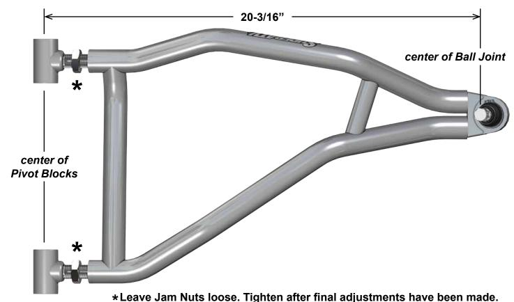
\* Leave Jam Nuts 100se. Tighten after final adjustinents have been made.
