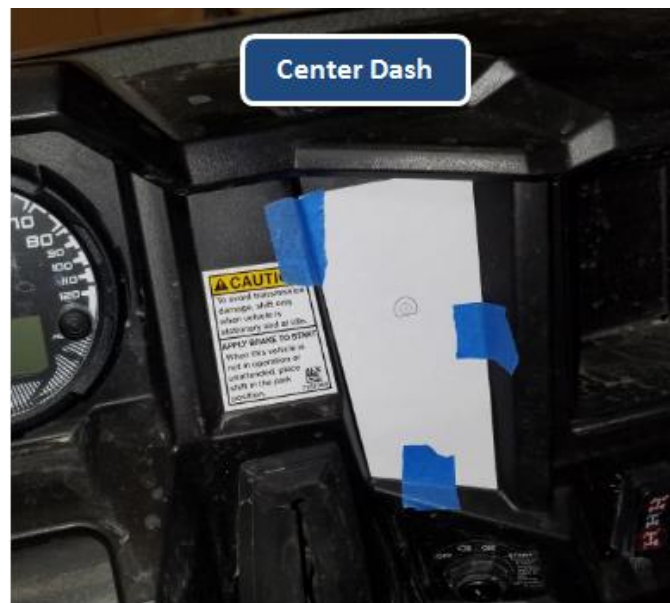
Figure 3 – Switch Mounting Location
