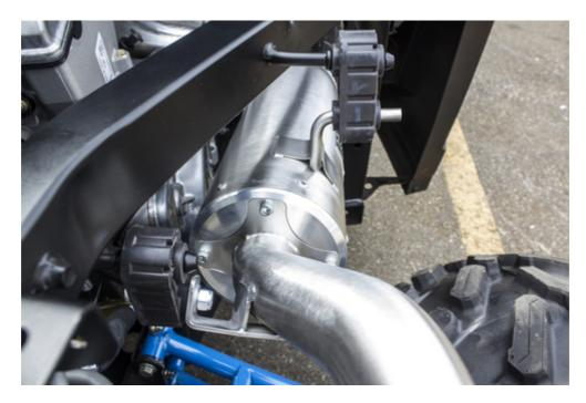
7. If equipped, plug the Oxygen sensor back into the wiring harness.
