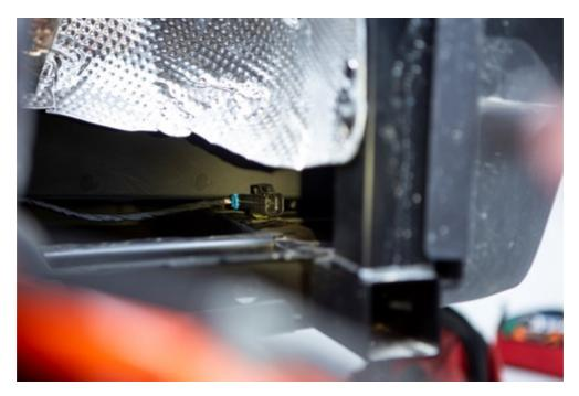
2. Remove the two bolts holding the rear portion of the exhaust to the head pipe. **Save the springs**, they will be used later during installation.
