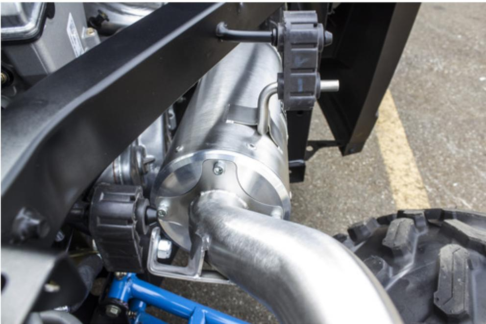
7. If equipped, plug the Oxygen sensor back into the wiring harness.
