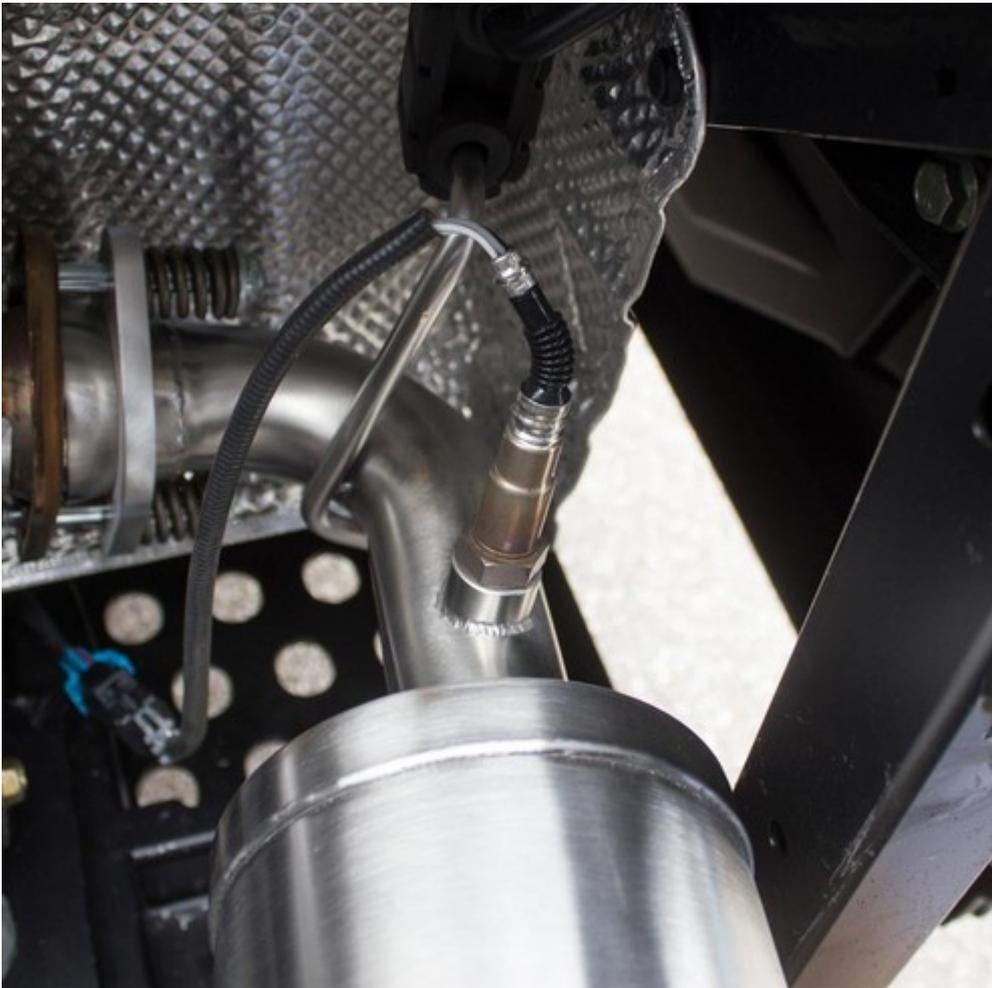
6. Using the remaining supplied hardware, mount the **tail pipe exhaust hanger** to the **bracket** on the **tail pipe**.
