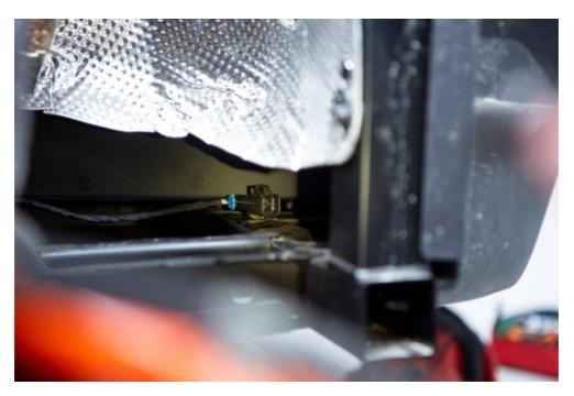
2. Remove the two bolts holding the rear portion of the exhaust to the head pipe. **Save the springs**, they will be used later during installation.
