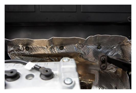
4. Disconnect the muffler from the three rubber hangers and carefully **remove the muffler**. Pay special attention to the oxygen sensor; do not let it, or the wiring become damaged while removing the exhaust, the wiring will have to be routed through the heat shield.
