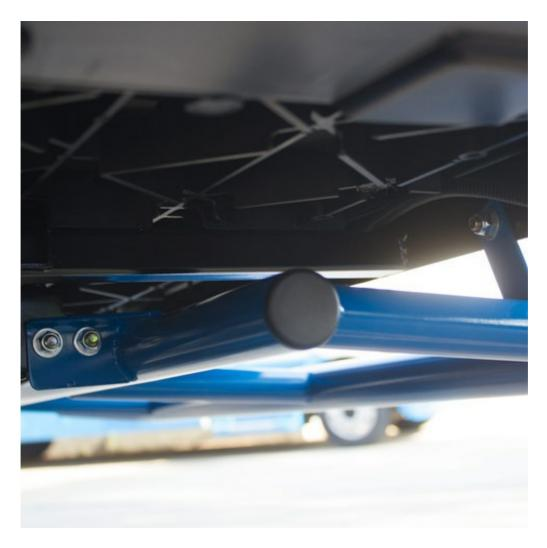
3. Check all areas around the bumper for proper clearance and alignment. Adjust as necessary.
