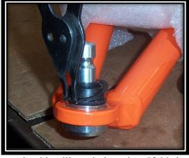
NOTE: If the ball joint is pressed in too hard it will crack the paint. If this happens then touch up paint can be applied.
