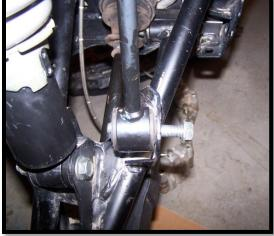
22. Reconnect the bottom of the shock to the upper arm using the stock hardware.
