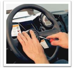
b) Using a ratchet, turn the steering nut counterclockwise. Continue this until the steering wheel locks at full turn, and then loosen the nut. **Do not remove the nut yet.**
