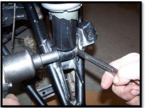
23. Reconnect the tie rod to the knuckle assembly.
