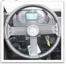
e) Now thread back on the steering wheel nut. Turn the nut clockwise until the steering wheel locks at full turn, and tighten the nut. Then replace the center cap.
