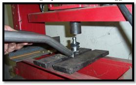
8. Reinstall ball joints into the NEW control arms.
