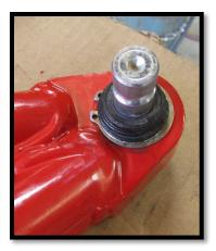
9. Now reinstall the bushings, sleeves, and pivot caps into the new arms. If you place some grease on them it makes the installation easier.
