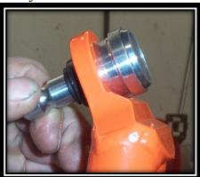
3. When pressing in the ball joint, support the ball joint end of the arm in a press with something solid below the arm and will allow the end of the ball joint to pass through completely. Be sure the support arm properly to allow the ball joint to pass through the hole straight and without interference. Again, be sure the boot will clear the fixture you are pressing into and the hole is deep enough for the full length of the ball joint to press into the arm.
