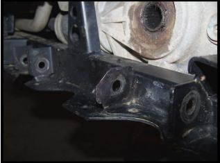
19. Use the factory nuts and bolts to connect the new upper control arms to the RUV frame.
