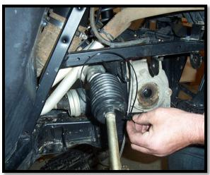
18. Before installing the new lower control arms, you will need to remove some material from the inner frame tab nearest to the axle. Remove just enough so the axle can clear the tab when it's at full droop. This is required on both driver and passenger sides.
