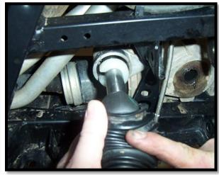
17. Pull boot back over the ball joint and steering stop and refasten with an (11" zip tie). Be sure to verify the zip tie is tight so prevent material from getting into the boot.
