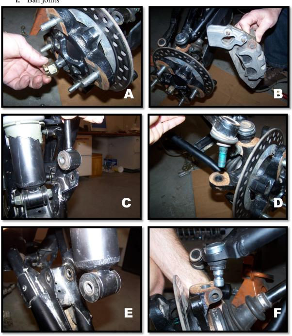
NOTE: When disconnecting lower ball joint from the knuckle assembly. You will need a 6mm hex key to hold the stud in place while removing the nut.
