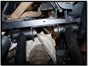
20. Reconnect the knuckle assembly to the ball joints.
