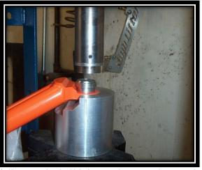
4. When pressing the ball joint, be sure to fully seat the ball joint so the snap ring can be fully seated. Make sure to clean the snap ring grove of any paint or material that may have become lodged in the groove during the press operation. We recommend you use a pick or fine point to clear the snap ring grove. Use a snap ring tool to secure the snap ring into place.
