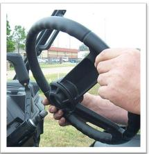
d) Now will be the time to adjust the steering wheel accordingly. Replace the wheel and make sure the wheels are turned back straight. The steering wheel should be straight up and down.
