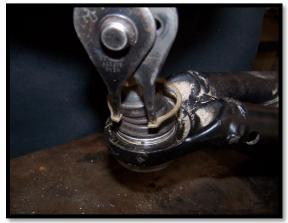
b. Using a press or a vise is suggested for removing and replacing the ball joints.
