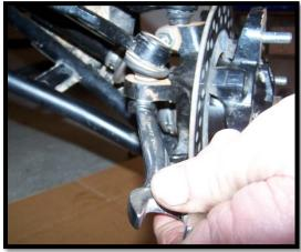
24. Reconnect the brake caliper and secure the brake line. Use the **8" zip ties** provided to secure the brake line to the new upper control arm.
