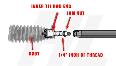
5. SET THE LENGTH OF THE NEW ADJUSTABLE TIE ROD TO THE MEASURED LENGTH OF THE ORIGINAL TIE ROD. DO THIS BY ADJUSTING THE TWO TIE ROD HALVES.
