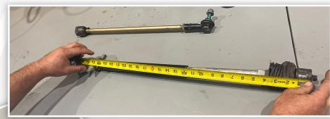
ONCE THE TIE ROD END AND THE INNER TIE ROD END ARE COMPLETED SET THE TIE ROD TO THE STOCK TIE RODS MEASUREMENT. NOW, USING AN ALLEN WRENCH SET THE FIRST SET SCREW ONCE IT IS ALIGNED ALONG THE CHANNEL ON THE TIE ROD AS SEEN IN THE IMAGE TO THE LEFT. NOW SET THE SECOND SET SCREW ON THE SIDE.
