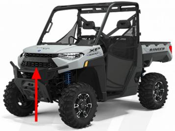
PLACE JACK UNDER THE CENTER OF FRONT AND LIFT UNTIL THE WHEELS ARE OFF THE GROUND. BE CAREFUL TO SECURE PROPERLY SO IT IS STABLE ON THE JACK OR JACK STANDS. REMOVE WHEELS.
