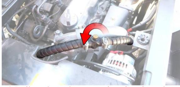
2. To achieve engine operating temperature depress the accelerator to increase The engine RPM. This will increase the preasure and flow of the water pump forcing more coolant through the heater. After operating temperature ceache turn of engine and open it. Trapped air should come out from heater system throughout bleeding valve.
