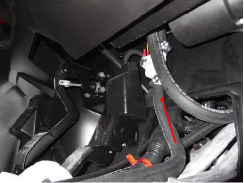
Install the short hose and remain of the hose to the heater tubes. Fix these hoses with the heater tubes by tightening straps and tighten these straps very hard. Insert the tightening strap onto the shorter hose and install elctromagnetic vent in same orientation like in picture. Tighten that strap very hard.
