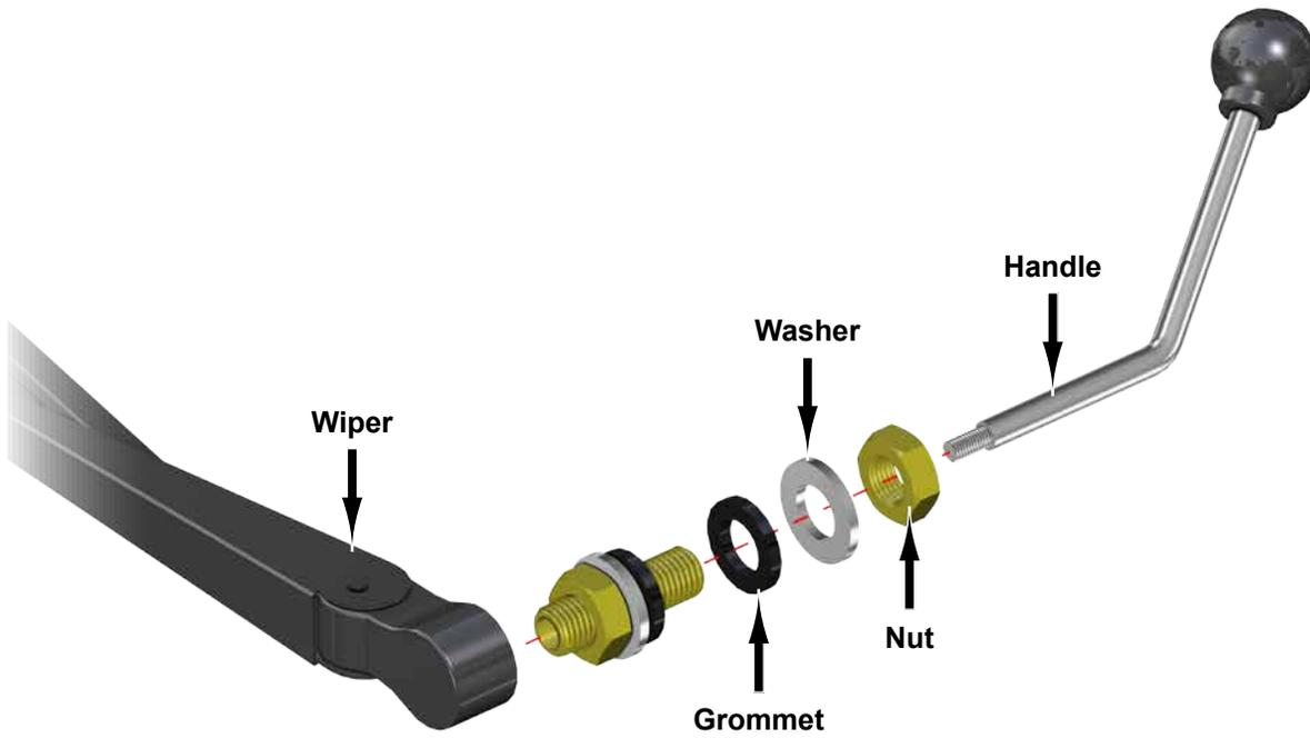
separate components shown from Wiper and assemble to Windshield
