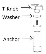
Remove the T-Knob and Washer from each of the Anchor Assemblies.
