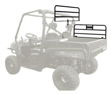
Place the Front Rail on the front of the Bed. Note that the slot is off-centered and that the slot should be towards the front of the Ranger.
