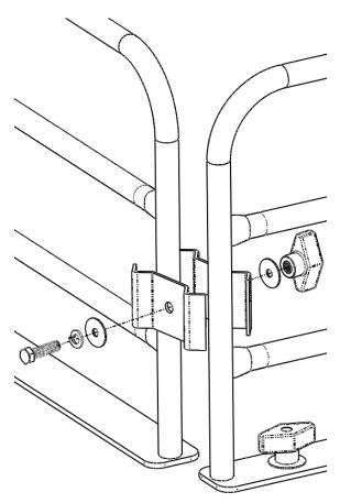
At both corners, place 2 of the Corner Brackets across the Front Rail and the Side Rail. Bolt together using the 5/16-18 Bolt with a Lock Washer and Washer on one side and a Washer and T- Knob on the other.
