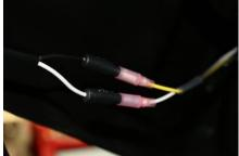
9. Lay the front small light harness out in the front under the hood, run the connector with the green wire to right side LED and run the connector with the yellow wire to the left side. Insert bullet connectors into LED connectors as shown above.
