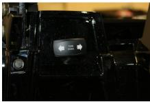
**Dielectric Grease** - Just like the OEM uses on their switches, we recommend using Dielectric Grease on all switch terminals, this keeps the water out, thereby reducing corrosion and helps increase reliability! Open the grease and put on the switch terminals and the connector terminals on both the Turn and Horn/Hazard switches, the more the better.
