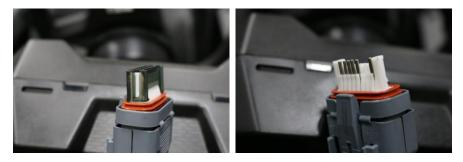
9. Remove Plugs – Using a pair of needle nose pliers remove the plugs from wire port 6 and 7, insert green wire terminal into 6 and yellow wire terminal into port 7.
