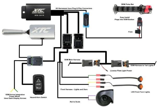
1. Remove the Hood and part of the dash cover. Mount the Control Module using the self-tapping screw provided.
